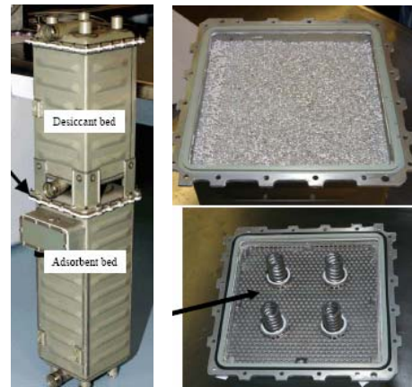
Figure 14 – Examples of ISS – CDRA packed granular beds and a spring-loaded ‘floating-lid’.
